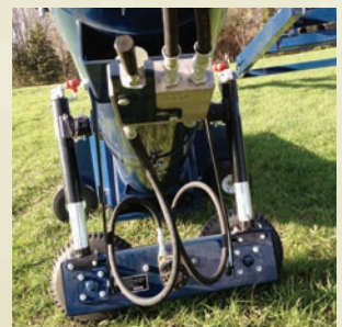
10" & 13" hydraulic wheel kit with double leveling jacks
